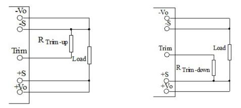
Connection for Trimming Up Connection of Trimming Down Resistance for trimming up :  $R_{Trim-up} = \left(\frac{21.5 \times 2.5}{\Delta V} - 15\right) (k\Omega)$ Resistance for trimming down:  $R_{Trim-down} = \left(\frac{(V_o - \Delta V - 2.5) \times 21.5}{\Delta V} - 15\right) (k\Omega)$
